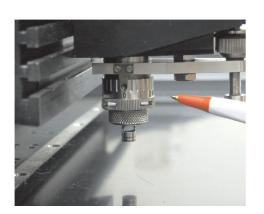
2. Place the carbide cutter in the rotary spindle (if you have not done so already). Tighten cutter by holding the pulley in one hand and screw the cutting tool knob counter-clockwise with the other hand.
