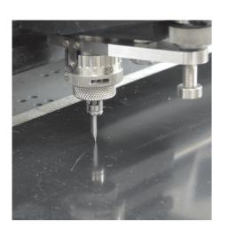
6. While the cutting tool is resting on the material, push the rotary spindle down until the nose touches the material. Both the cutting tool and the spindle should be touching the material.
